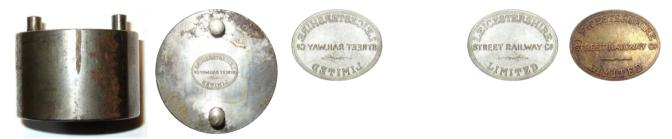
The die is cylindrical, diameter 64.6 mm, height 50.2 mm, with a very smooth outer surface. Two steel dowels protrude from the die face to locate opposing die. This is the obverse die of a fantasy token listed as Leicestershire 451YA in Smith and Smith<sup>(1)</sup>.
