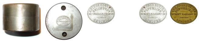
The die is cylindrical, diameter 64.2 mm at the die face and 64.3 at the base, height 47.3 mm, with a rough lathed outer surface and a small step at half height. Two holes are present to receive dowels from the opposing die. This is the obverse die of a fantasy token listed as Stoke-on-Trent 730YA in Smith and Smith<sup>(1)</sup>.
