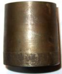
The die has a cylindrical base with a very smooth outer surface, 64.6 mm diameter. This has been lathed to taper to 59.8 mm at the die face. The die is 71.5 mm high. This is a plantation token of the Dutch East Indies (LaBe 87<sup>(3)</sup>, LaWe 96<sup>(4)</sup>) and has been listed as a pattern in the most recent catalogue, even appearing on the front cover<sup>(3)</sup>. All known specimens of the token are uniface.
