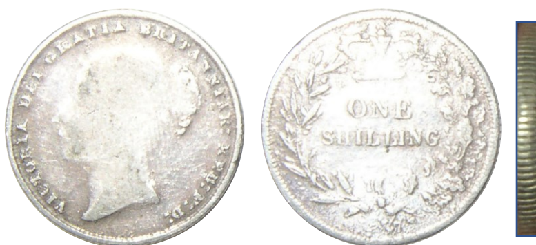
Fig. 4. Counterfeit 1877 shilling. Unusual material, very worn, traces of plating. Very good edge milling. 200%. 5.490 g, 23.52 mm, 180°.
