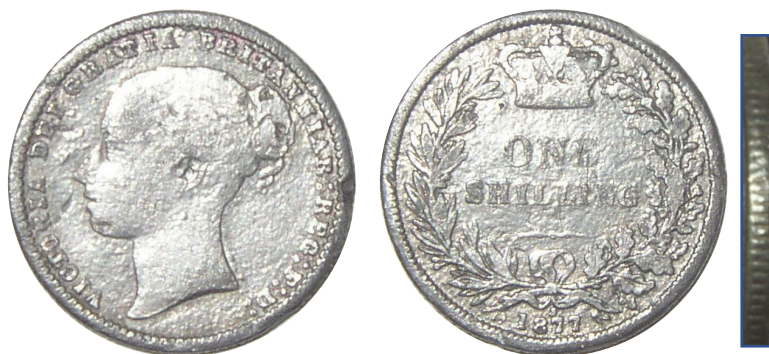
Fig. 2. Counterfeit 1877 shilling (die number 3). Typical cast white metal. Edge a bit rough from the cast. 200%. 3.995 g, 23.56 mm, 180°.
