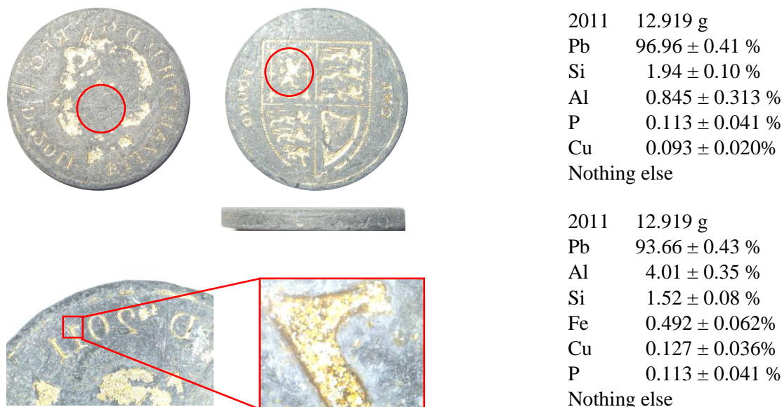
Fig. 6. Analysis of a 2011 incuse counterfeit.
