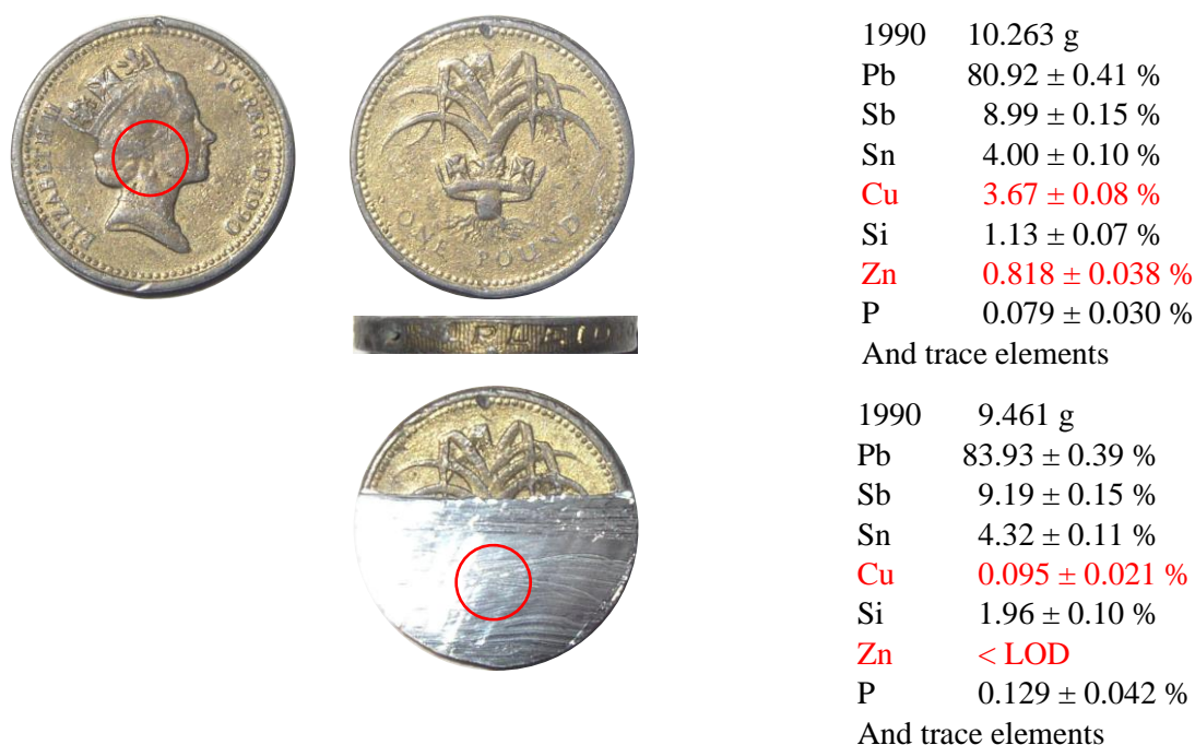
Fig. 4. Analysis of a 1990 coated lead alloy counterfeit.
