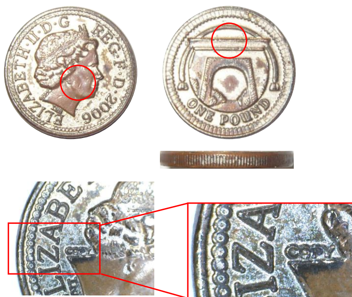
Fig. 5. Plated copper/brass counterfeit from false dies.
