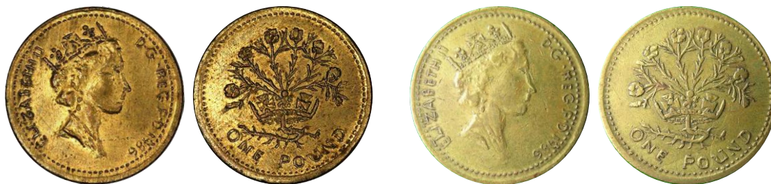
Fig. 6. Counterfeit round pounds struck in brass from hand cut dies (2,3) .
