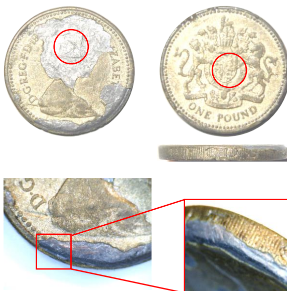
Fig. 1. Lead core with a metallic resin coating. DECUS edge. Probably 1983. 150%.
