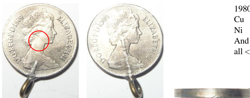
Fig. 4. Counterfeit made from a 1979 and 1980 5 pence.
