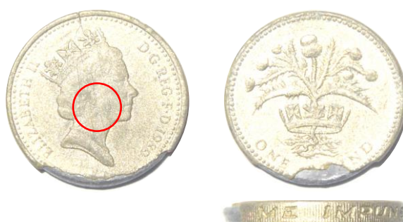
Fig. 2. Lead core with metallic resin coating. NEMO edge. 1989.
