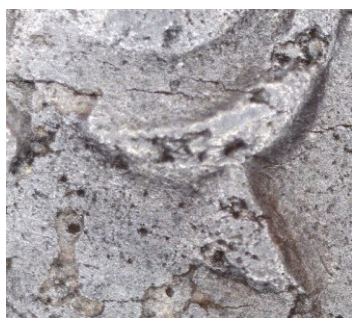
Type 1a with triangular flaw.
