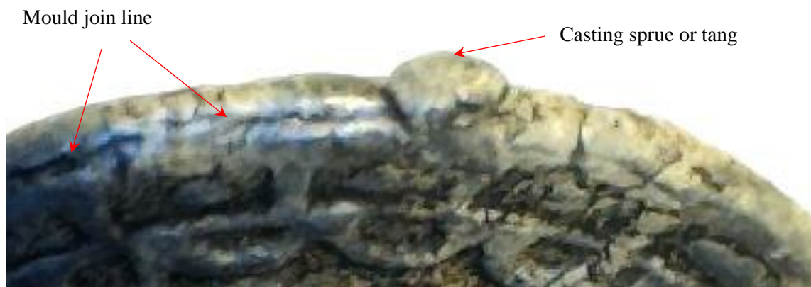
Fig. 3. Casting sprue and mould line on edge of token #004.
