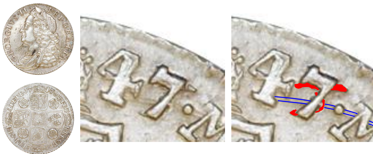
Fig. 1. 1747/6 shilling with close-ups. Overdate in red, a die scratch/flaw in blue.
