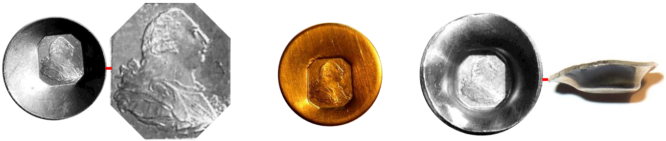
Fig. 3. Testing the punch in pewter (with close-up), brass and a larger force in pewter.
