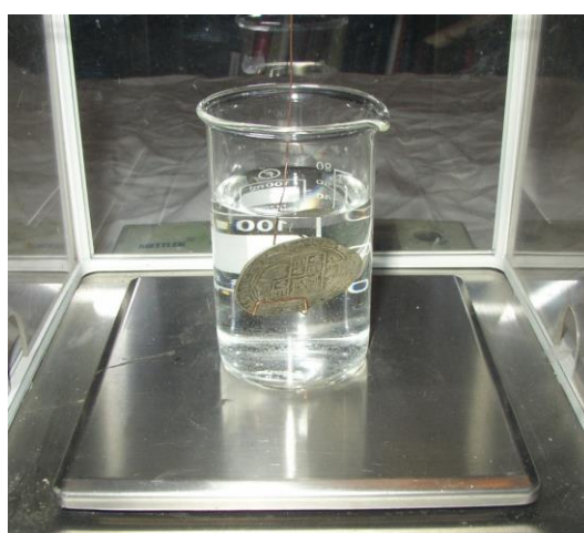
Fig. 4. Measuring the buoyancy force on the submerged coin.
