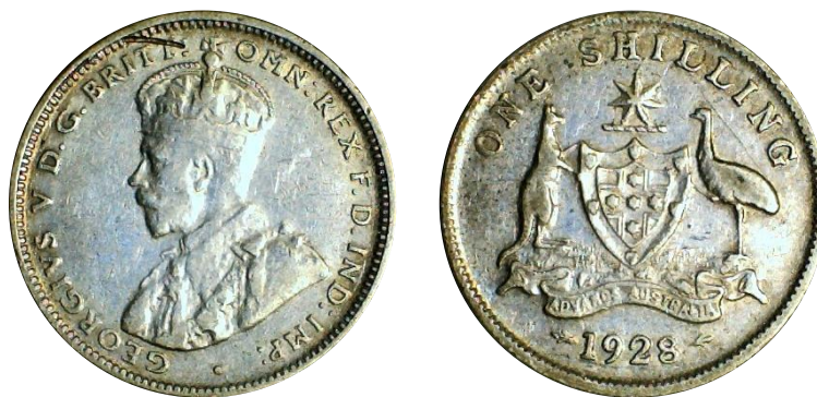
Fig. 1. Australian counterfeit from 1928. 23.82 mm, 5.651 g, XRF metals: Ag 93.0%, Cu 5.2%, Sn 0.5%, with other contaminants. (Shown 200%).
