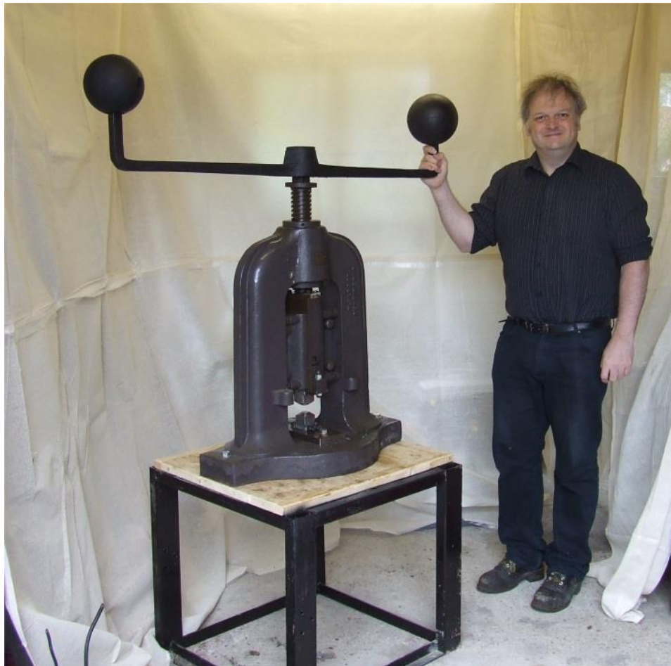
Fig. 7. Screw press ready for use.
