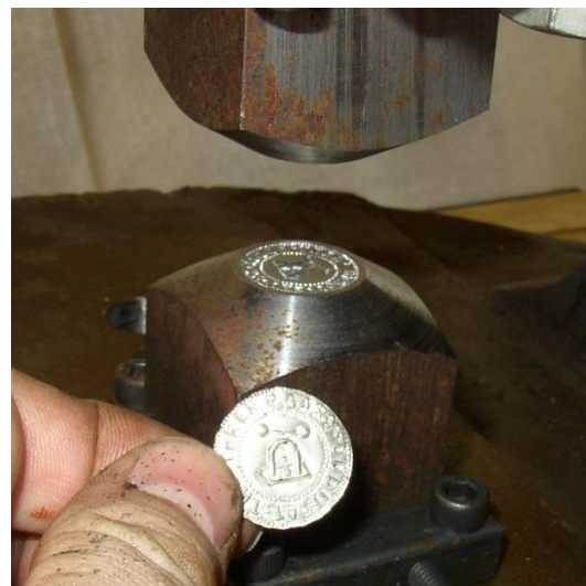
Fig. 7a. First test on pewter blanks.
