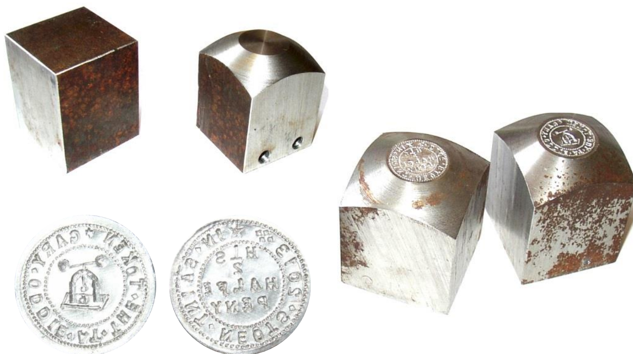
Fig. 5. Creating new dies and close-up of finished die face.
