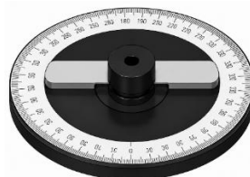
A simple calibrated turntable made for less than £10
